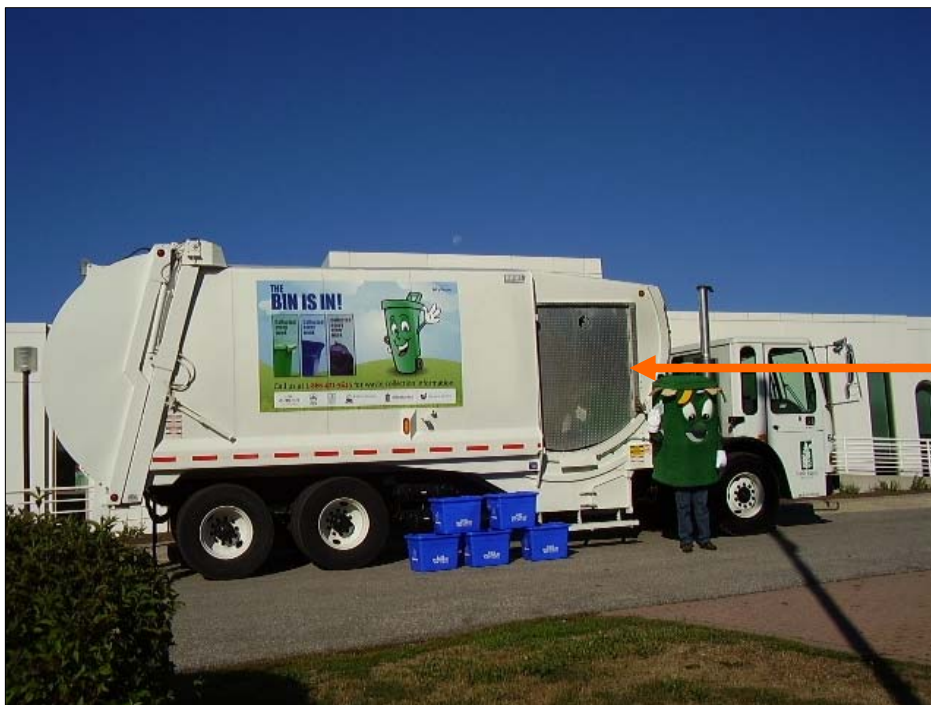
Figure 8: King side load compacting co-collection truck for recycling and organics
