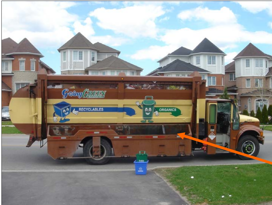
Figure 7: Richmond Hill over the top side loader collection truck for recyclables and organics
