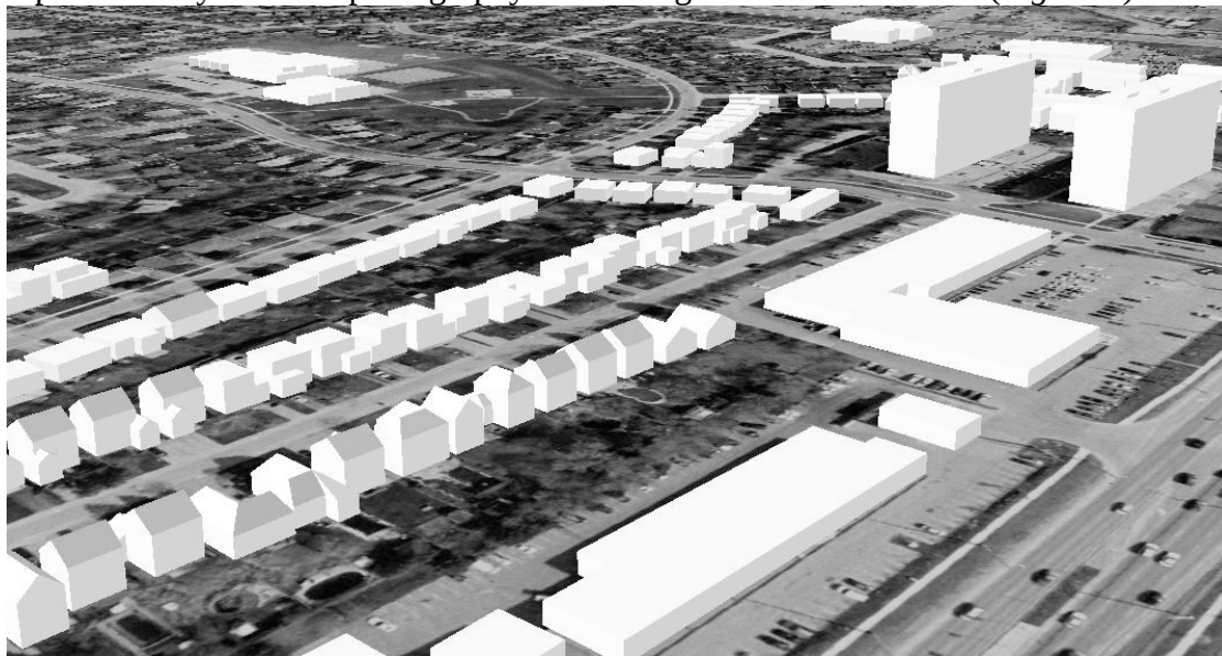
Figure 1 Building footprints extruded as buildings: Simple Urban 3D Model Newmarket Centre In Stage 3, building façades can be added to the model from photos of the actual buildings or from architectural designs and master plans to create a photorealistic model
