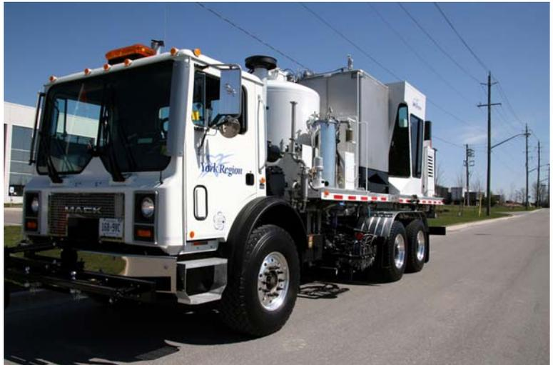
The line-painting truck is low-emission and runs on biodiesel fuel. It is capable of applying lines in white or yellow, in a solid pattern, broken pattern or combination of the two. Additional features of the paint truck include:
